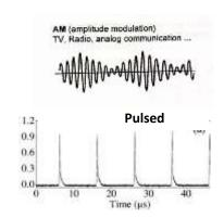
Today, nearly all signals are digital—meaning the signal is zero in amplitude (i.e. strength), except when it is a strong, very short pulse, essentially the antithesis of an analog signal. Average measurement designed for analog signals of yesteryear cannot "see" digital signals.
